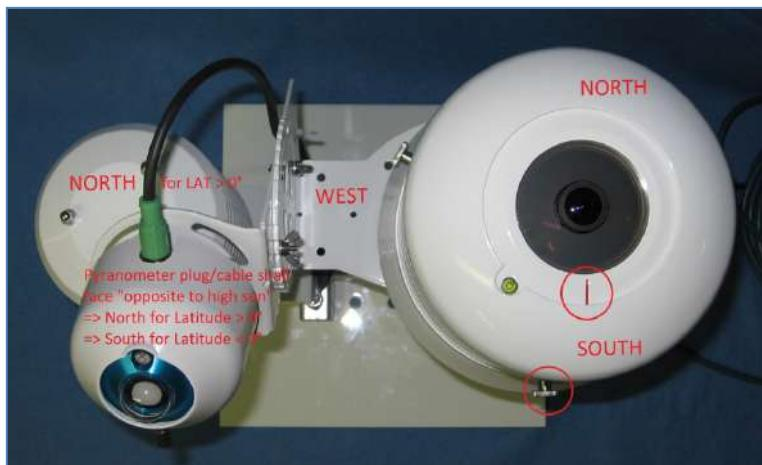
When mounting the Pyranometer, consider Northern or Southern hemisphere. The plug and cable always shall face "away from sun", to avoid heat by exposure to direct sun radiation, therefore likely corrupt Pyran irradiance data.
