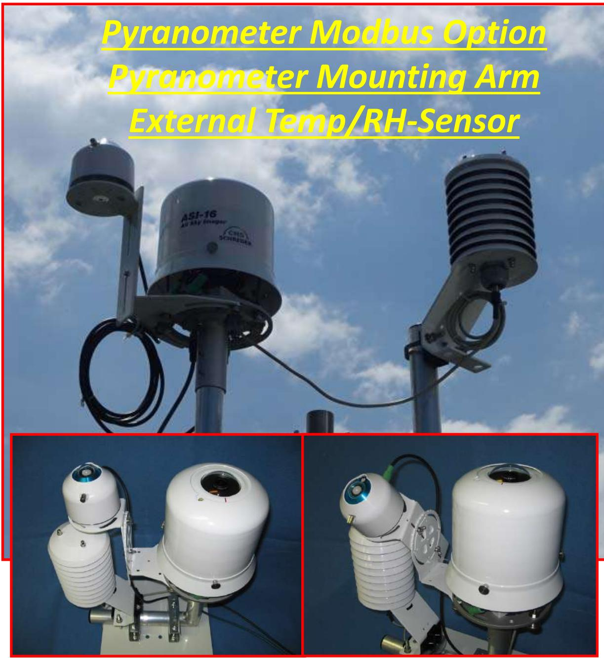
Pyranometer Option: To connect and operate a Modbus Pyranometer with any new ASI-16/5n, for logging of real-time irradiance data (Act, AvP, AvM, Min, Max). Subject to purchase of ASI Pyranometer Option. - Activation after Purchase.
