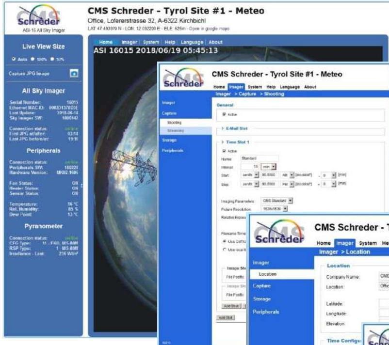
Client Site Location (Lat/Lon/Ele), stored into each JPG EXIF dataset. JPGs upload to (S/FTP(S) storage. Temporary local storage in case of FTP server or network problems. JAVA-based maintenance tools.
