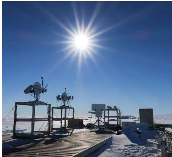
An elite solution for high-precision solar radiation measurements, the STR-21G-S1 and STR-Series sun trackers are designed for solar energy research, photovoltaic system performance monitoring, and meteorological applications. It is suitable for any application that requires the highest standards of accuracy and reliability.
