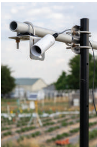
Commercial-Grade (SIL-4H1) 32° horizontal; 13° vertical Commercial-Grade (SIL-111/411) 22° half-angle
