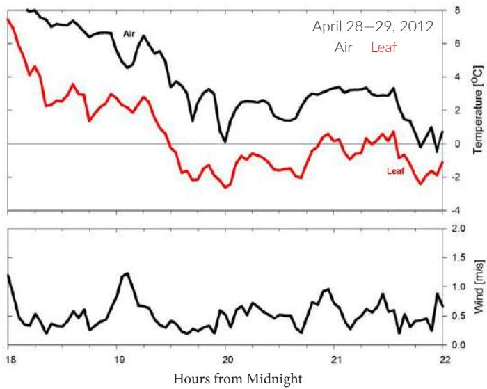
Leaf temperature approximations measured with an Apogee SF-110 compared to air temperature (top panel) and wind speed (bottom panel) on the evening of April 28, 2012. Leaf temperatures were below air temperature after 8 P.M. and reached freezing 6 hours before the air temperature.
