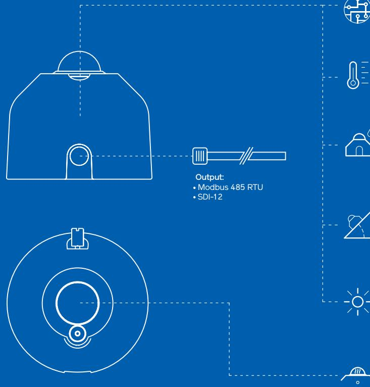
Smart electronics: signal transducer with x2 different digital outputs.
