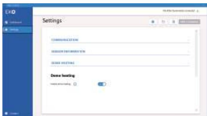
The simple ON/OFF toggle gives users complete control over the dome heating function.
