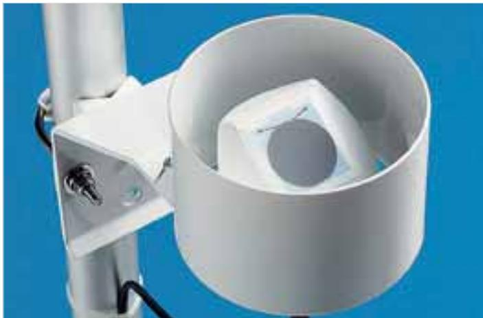
intensity. The ON/OFF output comes with a delay circuit that indicates the "rain over" condition with a 2 minute delay, so that the "rain over" condition is distinguished from the "light rain" one. The heater can be disabled when power consumption is critical. To do it, set the Heater OFF input on OV. If requested when ordering, a bird spike, consisting of a 6-spoke ring (spike height: 60mm, diameter: 3 mm), can be mounted.
